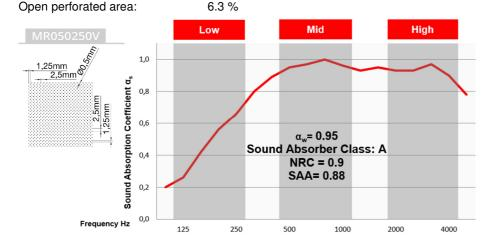
Through the combination of the finest stamping technology and MDF-cores Acoustic-CompactBoard<sup>®</sup> products offer superior sound absorption properties.
