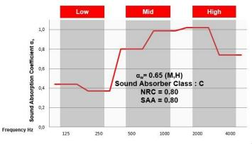
Due to the combination of absorptive material and reflecting design surfaces, Acoustic-RibPanels are a quick way to optimize room acoustics in style.
